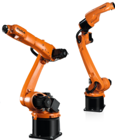
KR CYBERTECH nano series Suitable for the entire range of applications, such as handling, welding, palletizing, assembly, bonding, measuring, etc.
