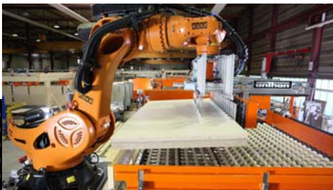
Mounted on a linear unit: the KR 1000 1300 titan handles wooden boards at Anthon.
