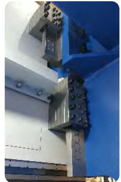
Beam movement on heavy-duty bronze sliders to secure safety and accuracy
