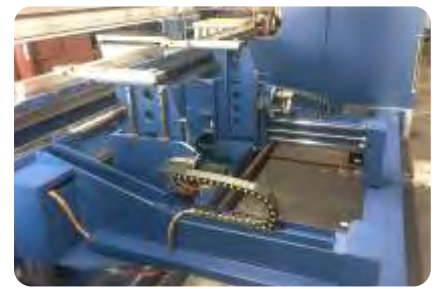
6-axis back gauge, X1-X2-R1-R2-Z1-Z2 (optional)
