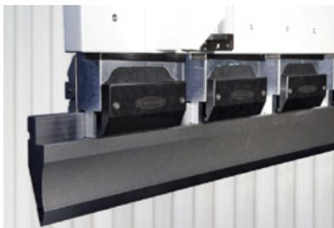
■ By the pneumatic clamping tools model WTC patented by Warcom, all PROMECAM tooling up to 20 Kg can be loaded from the front side. WTC moves up and block automatically the punch giving a perfect self alignment.
